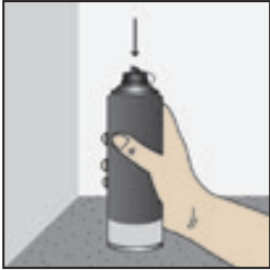
Push the applicator nozzle firmly into place without pressing the trigger or the valve.
