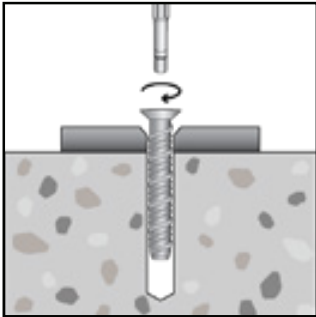
Insert anchor into hole and screw in using hand or power tool to drive the driver bit. Apply constant forward pressure when driving and tighten to the specified torque.
