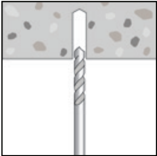
Drill hole into substrate to the specified depth
