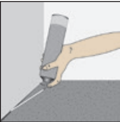
Invert can and gently apply pressure to the top of the actuator to extrude. Apply foam in layers, allowing time between layers for expansion. Lightly mist with water between layers.
