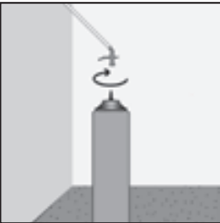
Screw the applicator nozzle firmly into place without pressing the trigger or the valve.
