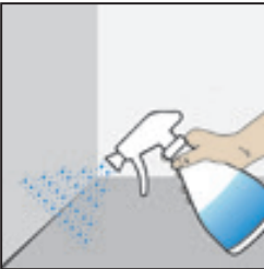
Lightly mist surfaces with water before applying foam to improve adhesion.
