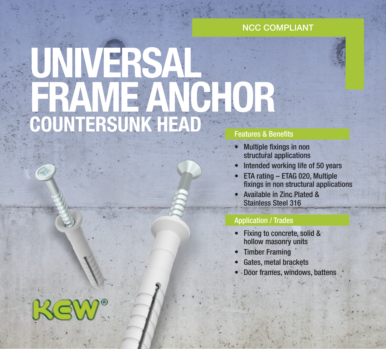
Available in Hex head and Countersunk head options
