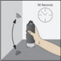
Shake can vigorously for 60 seconds before use. Repeat periodically during use.
